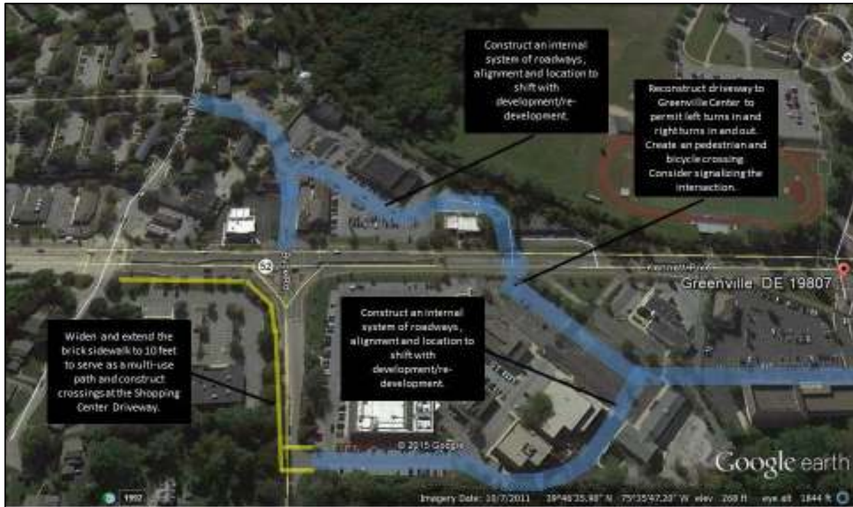
Figure 7-6: One possible way to connect Greenville Crossing, Powder Mill Square and Greenville Center with a system of roadways following the current parking patterns.
