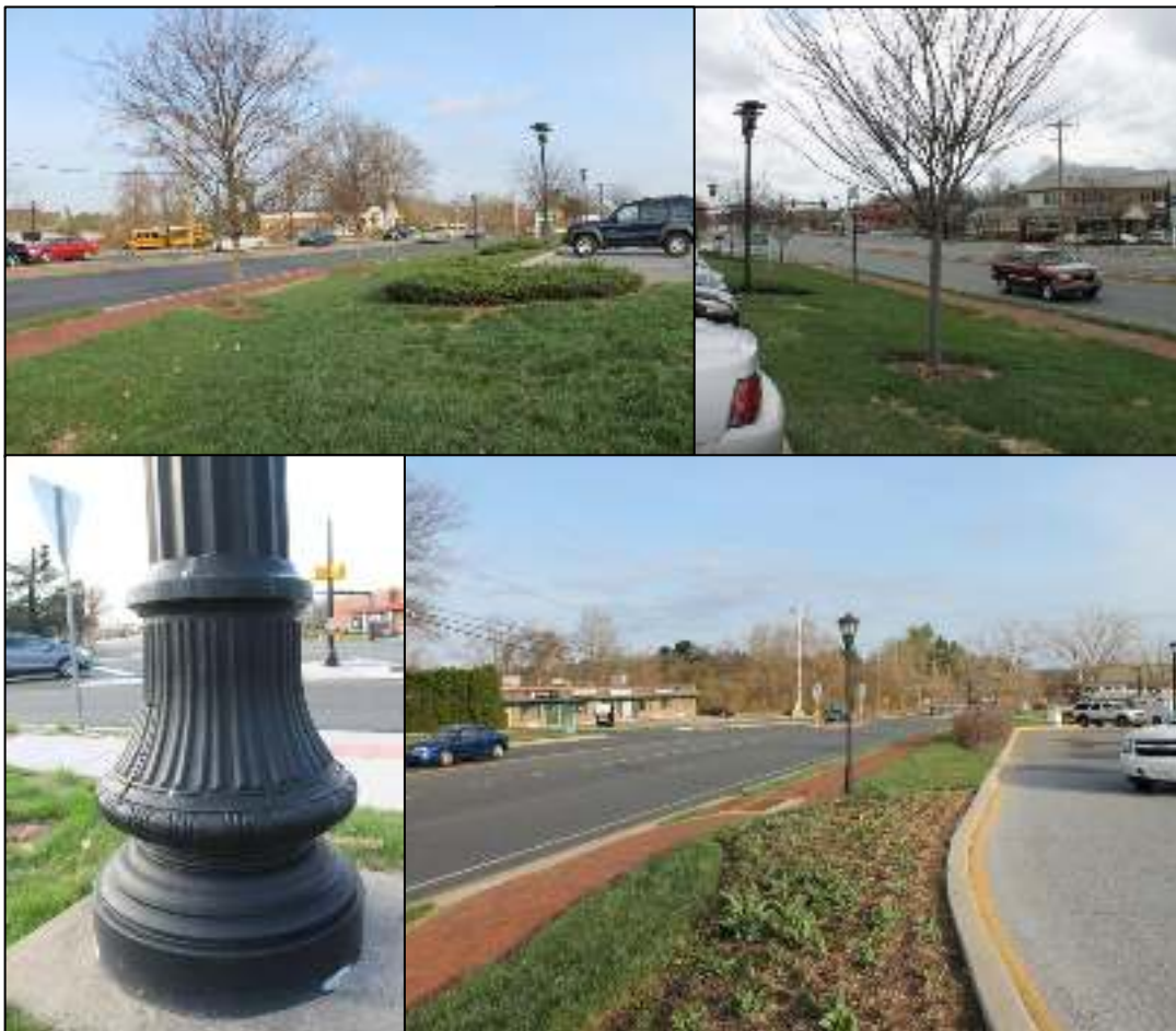
Elements of context sensitive design installed by DelDOT in conjunction with the community. Note the brick sidewalks, the ornamental light poles and the landscaping along the street.
