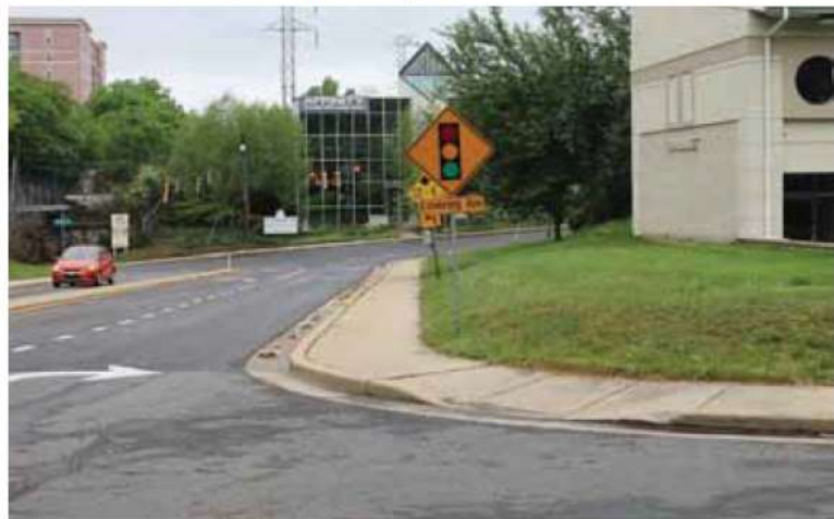
Figure 7: The suggested multi-use side path would require extending sidewalk into the grassy right of way along the north/west side of Augustine Cut Off between Wawaset Street and Lovering Avenue
