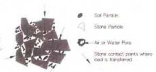
Fig. 1: The stone lattice bears loading while the soil particle partially fills the lattice voids.
