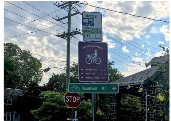
Figure 35. MUTCD compliant bicycle wayfinding signage
