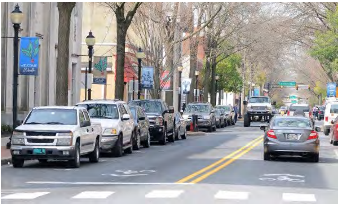
Figure 15. Sharrows on W. Lockerman Street in Downtown Dover, courtesy Delaware State News
