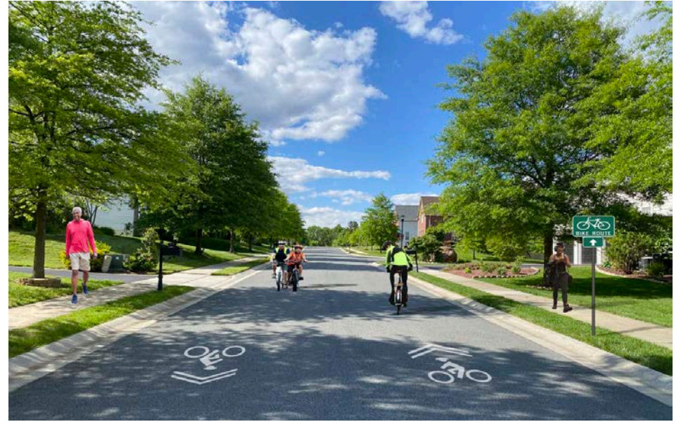
Figure 25: Photo sketch of signed shared lane markings on Chariot Road with existing sidewalks in Greenville Overlook development for alignments B1 and C1
