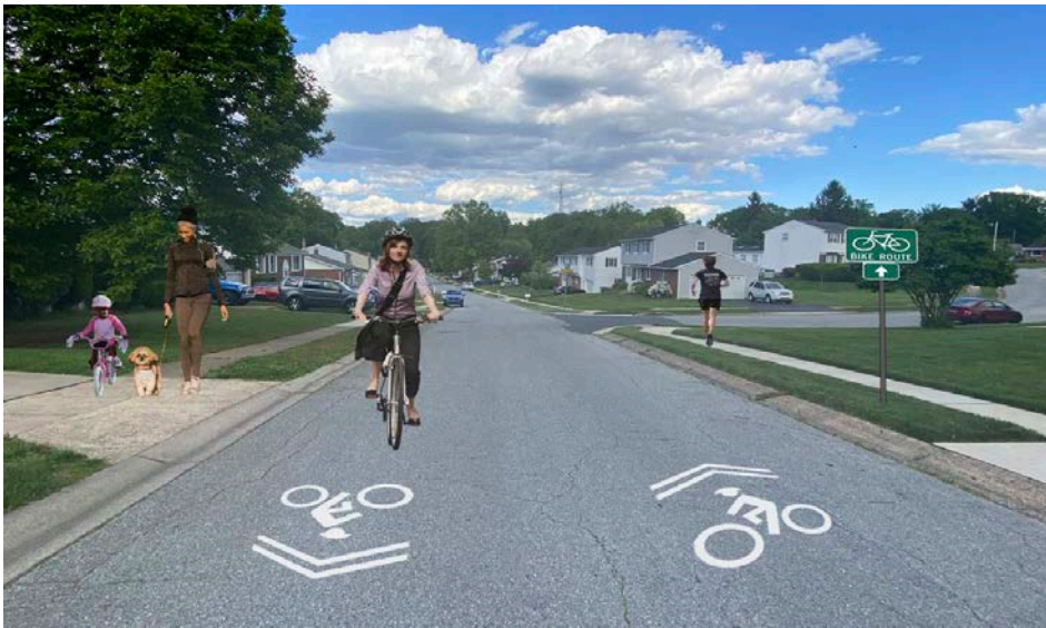
Figure 10: Photo sketch showing signed shared lane markings on Crossgates Road with the existing sidewalks
