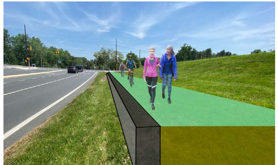
Figure 14: Photo sketch of shared use path between Millcreek Road and existing stormwater management facility that may require a retaining wall
