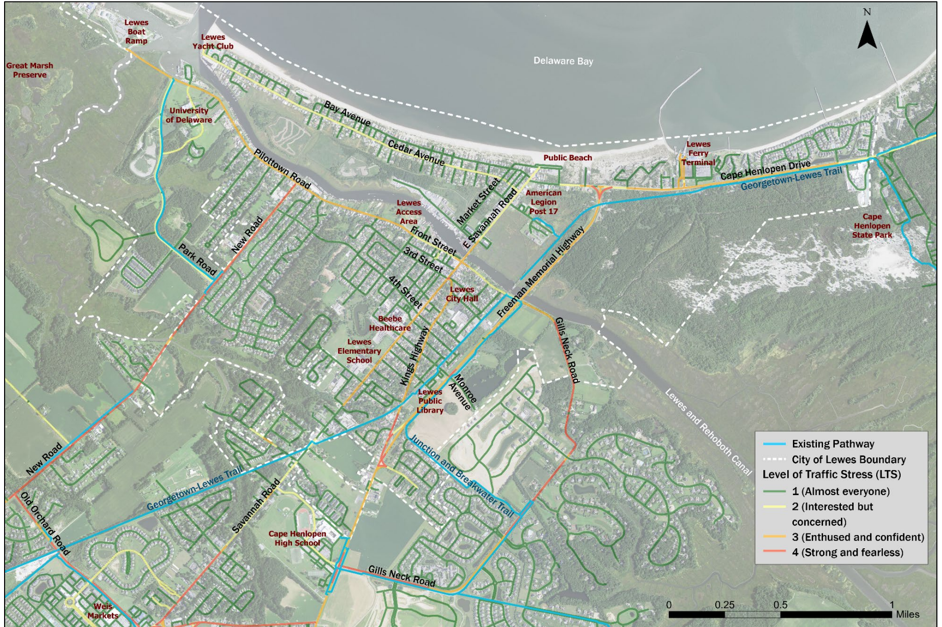
Figure 5. Bicycle Level of Traffic Stress and existing pathways in the Lewes area
